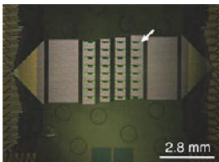
Fig. 15. Image of magnetonanosensor chip with 64 sensors in an 8 x 8 array. The arrow indicates a single chip. [Adapted from Gaster et al., 2009]
