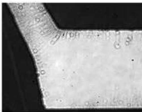
Fig. 9. CNT (0.2 mg/mL) enhanced collection of E. Coli bacteria ( 10^5 CFU/mL) (Zhou et al. , 2006). Reused with permission.
