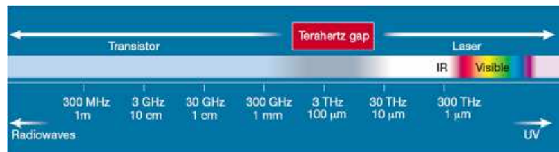
Fig. 3.1. The THz gap. The gap, lying roughly between 300 GHz and 30 THz, exists because the frequencies generated by transistors and lasers, typical semiconductor devices, do not overlap. No current semiconductor technology can efficiently convert electrical power into electromagnetism in this range
