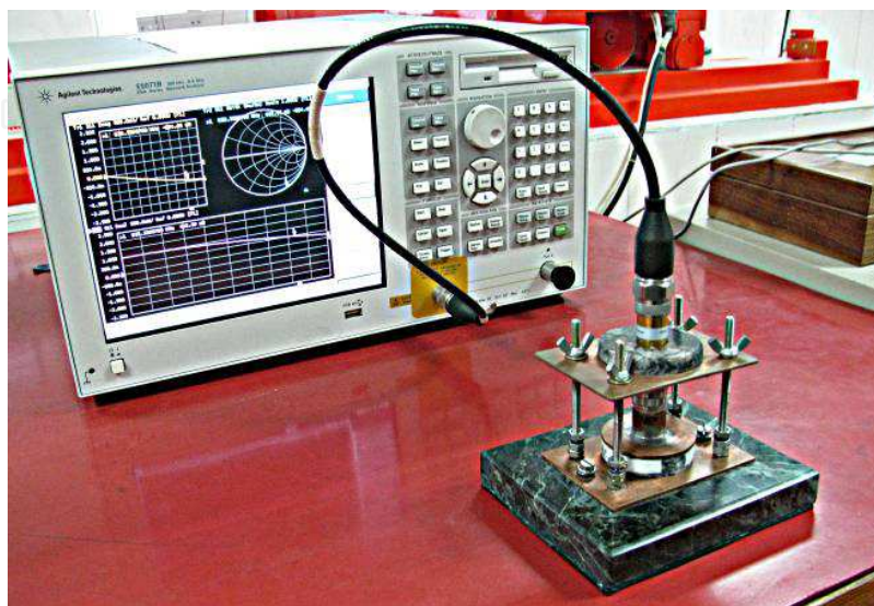
Fig. 4. VNA and the rock sample holder
