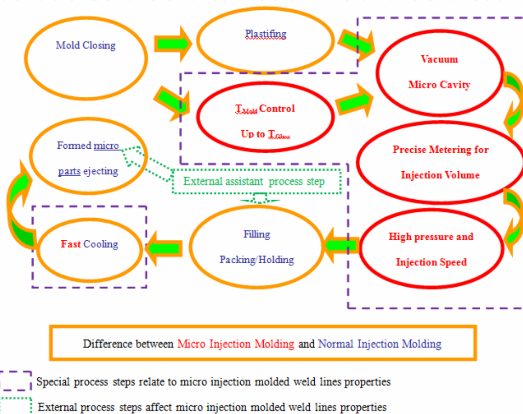
Fig. 1-2. Micro injection molding processing steps
