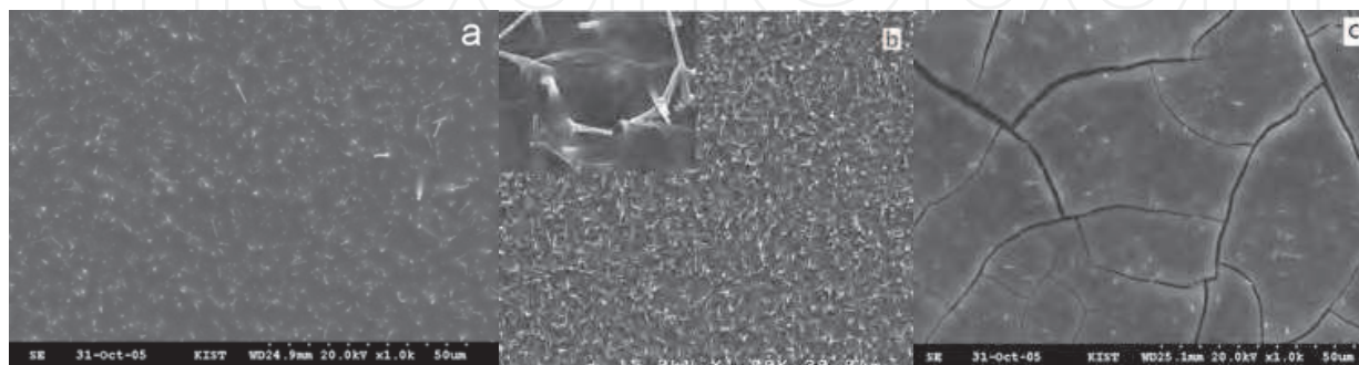
Fig. 2.7 SEM images of (a) SiNW-ErAlO (Ren, 2008), (b) SiNW-ErSiAlO (Si/Al=3/1) (Ren et al., 2007a) and (c) SiNW-ErSiO (Ren, 2008).
