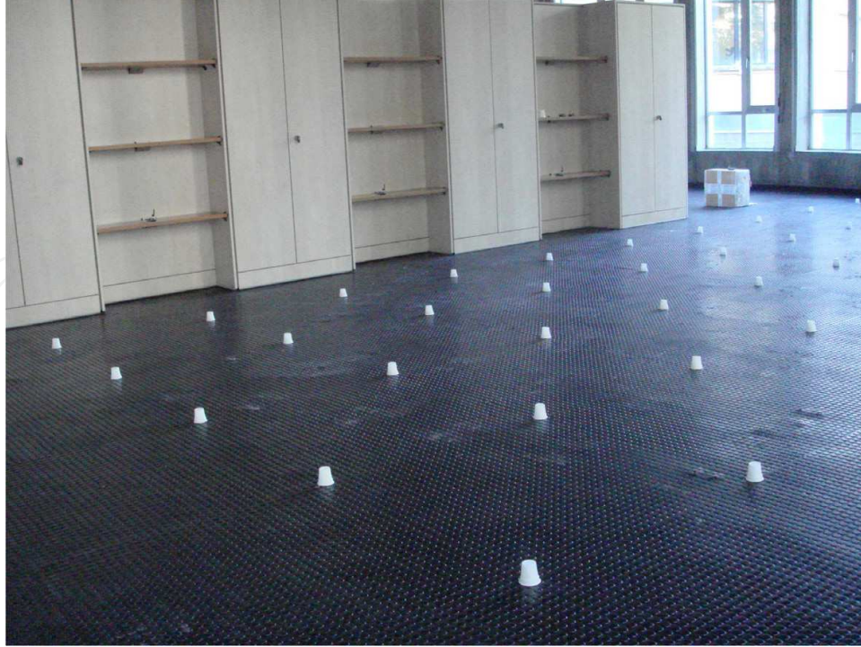
Fig. 7. Deployed testbed using CrossBow's MICAz sensor nodes for ranging calibration.
