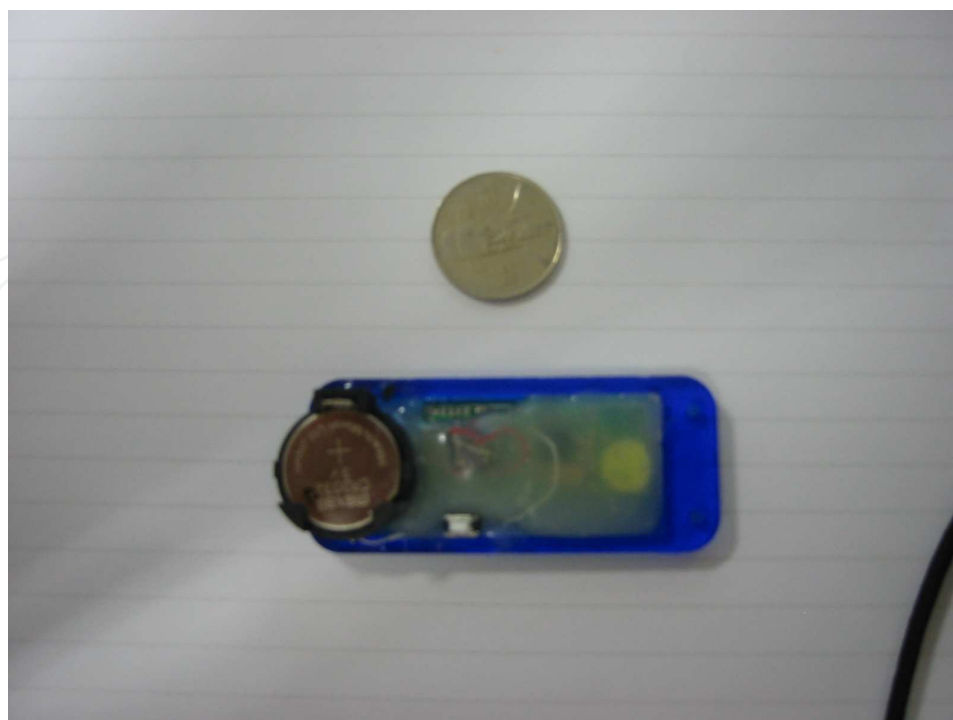
Fig. 2. The size comparison of wireless accelerometer sensor module
