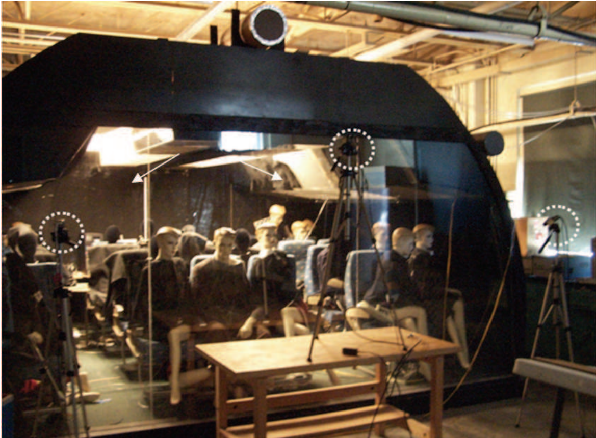
Fig. 24. Experimental aircraft cabin. Cameras positions are marked by white circles. The two ventilation inlets are marked by white arrows.
