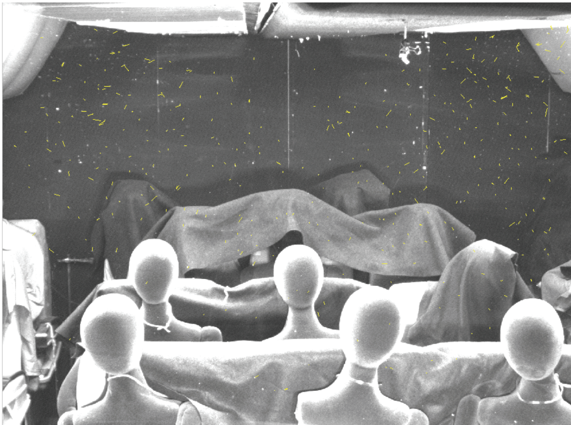
Fig. 26. Instantaneous 2D velocity in the aircraft cabin using the fast normalized cross-correlation temporal tracking scheme. Vortices due to recirculation of the air in the cabin can be seen over the aisles. University of Illinois at Urbana-Champaign, Department of Agricultural and Biological Engineering, Bioengineering Research Laboratory, USA
