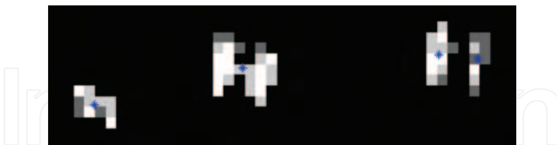
Fig. 10. Output of the center of mass calculation by weight averaging on three particles of the same image. Far left and center particles yield one centroid whereas far right particle displays two disconnected local maximum and therefore yields two centroids
