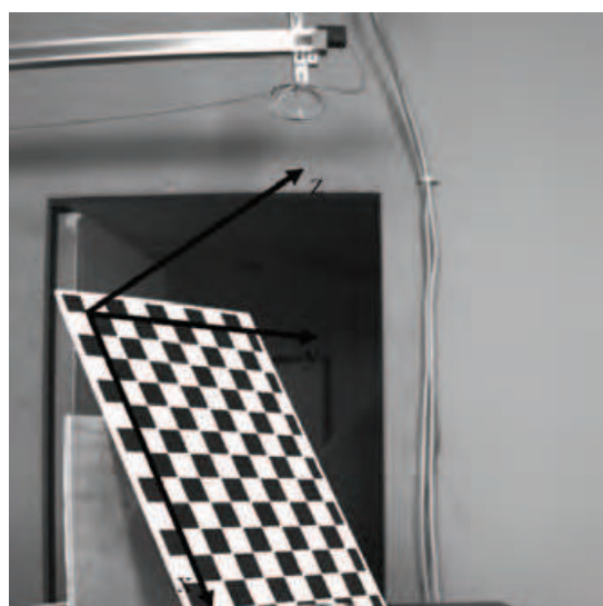
Fig. 14. Calibration target as observed from camera 2 viewpoint.
