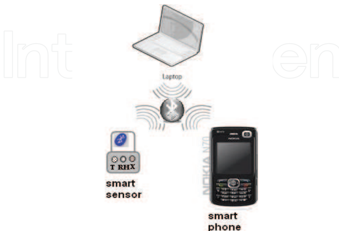
Fig. 10. Air quality virtual measuring system's architecture based on a smart sensing node (SN) with Bluetooth communication capabilities, and on a smart phone
