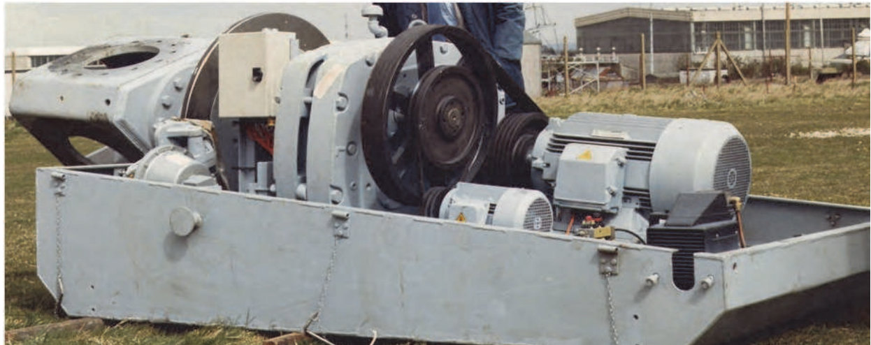
Fig. 16. Drivetrain of the Windharvester wind turbine.
