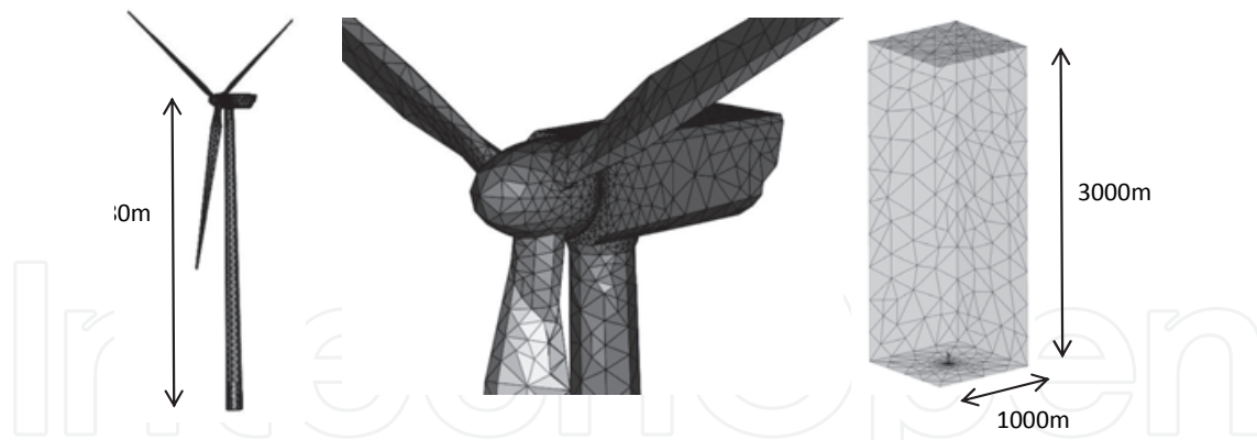
Fig. 11. A typical model of a turbine used in the research. The size of the analysis volume is considerably larger than the turbine, in this case 1km x 1km x 3km.
