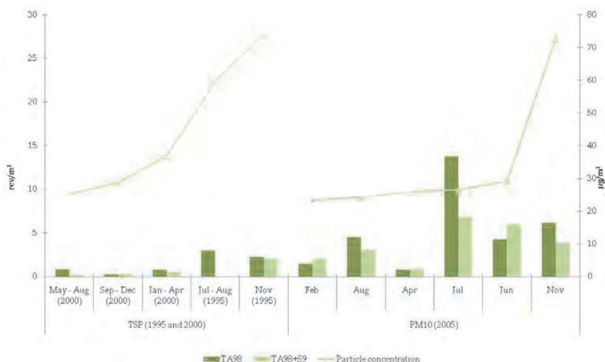
Fig. 3. Mutagenic activity of airborne samples evaluated by the Salmonella /microsome assay for TA98 strain (revertants/ \text{m}^3 ) in Triunfo in an area under the influence of a petrochemical complex ordered by TSP, or PM10 mean concentrations ( \mu\text{g}/\text{m}^3 ). -S9, +S9, absence, presence of S9 mix fraction.
