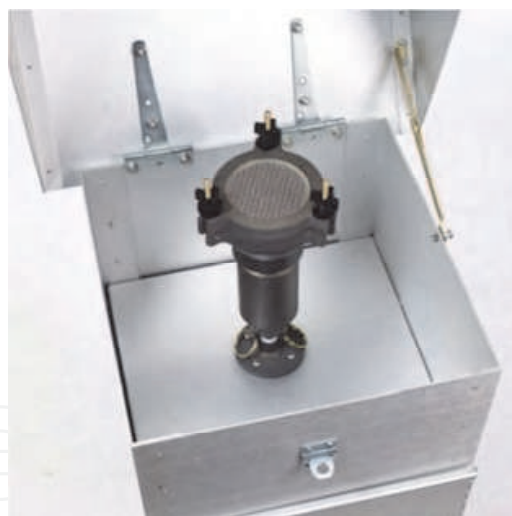
Fig. 2. Head of a PUF (polyurethane foam) sampler.
