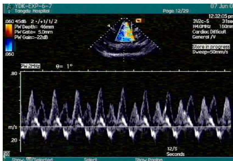
Fig. 21. Doppler signals generated by fluid and tubing motions. The frequency of the motion of the tubing and the frequency of the peristaltic pump were varied. The frequencies of two motions were very close, but desynchronized. The relative magnitude of the measured signals during the cycle varies even though the actual frequencies and velocities of motion and flow were constant. The two motions may have various phase combinations, yielding different modified Doppler flow velocity spectra
