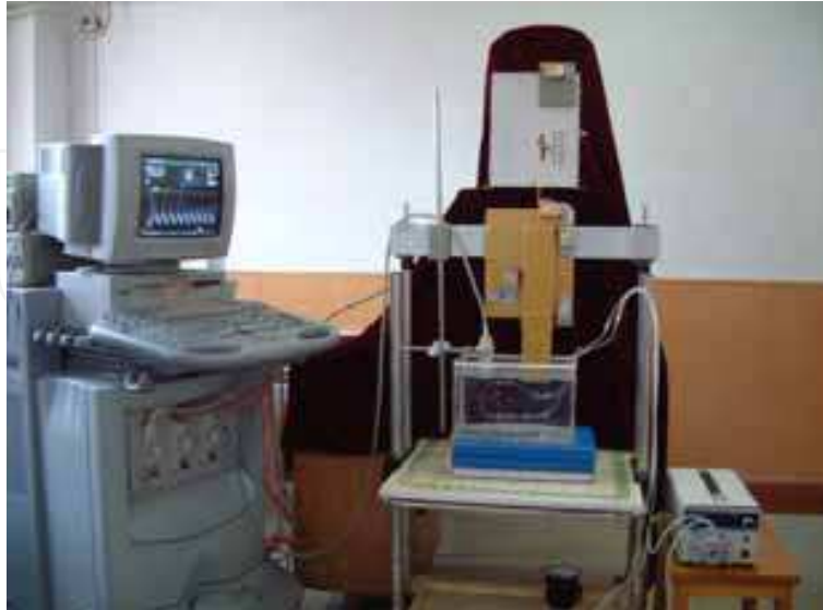
Fig. 1a. Photo of the whole set of the in vitro model experiment. From the right to the left of the photo the whole set is displayed. Right: the perfusion pump which drives the simulated blood in the tubing; Middle (from top to the bottom): the top is the TD-4 cardiac motion simulator (specially designed and home-made) that moves the plastic board up and down; the middle is the gears and connectors that connects the plastic board below; the bottom is the water tank with the plastic board in it. The tubing with 5% fiber-water slurry, the simulated blood, is fixed on the plastic board that is connected with the connector above. The plastic board with the tubing may move up and down freely by the simulator. The echo transducer is separately fixed on the frame of the setup; Left: Ultrasound machine, Sequoia 256
