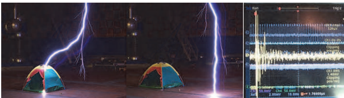
Fig. 15. Left : Basic structure of the tent as a model for the Faraday cage. There can be arcing if some metal is present inside the tent (no lightning safety), Mid : Lightning event occurs near the object due to slight moment of the electrode. Right : The measured electric field due to arcing (impact) of the lightning discharge on the model of Faraday cage.
