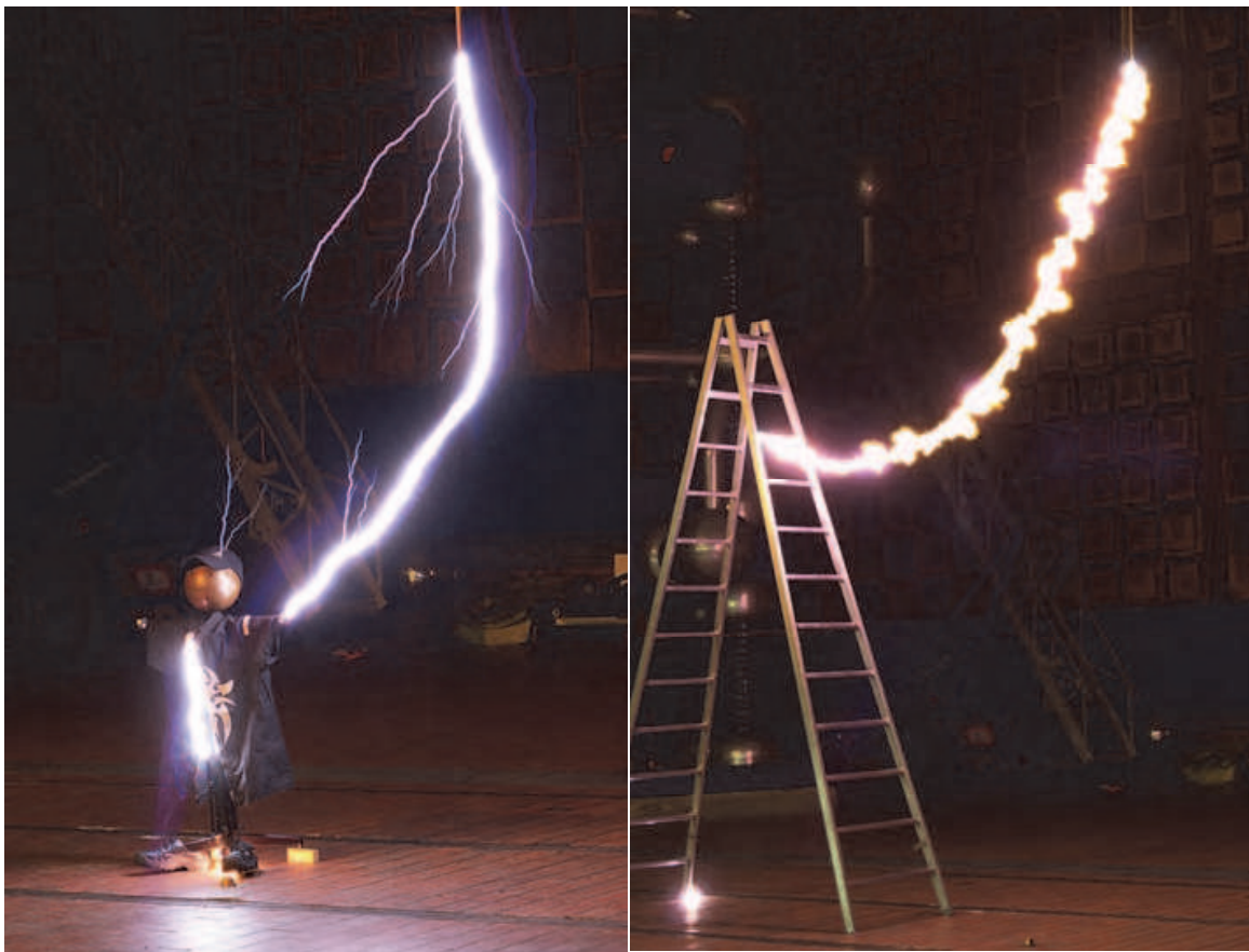
Fig. 13. Left : Lightning event occurrence on a model. Also branched lightning (to ground and air) was observed. Right : Color changes (intensity) due to discharges along the rope. The variations indicate current interaction with fibers of the rope under impact of lightning discharge of \sim 1.8 MV. Post-event inspection revealed no damage in the rope, macroscopically.
