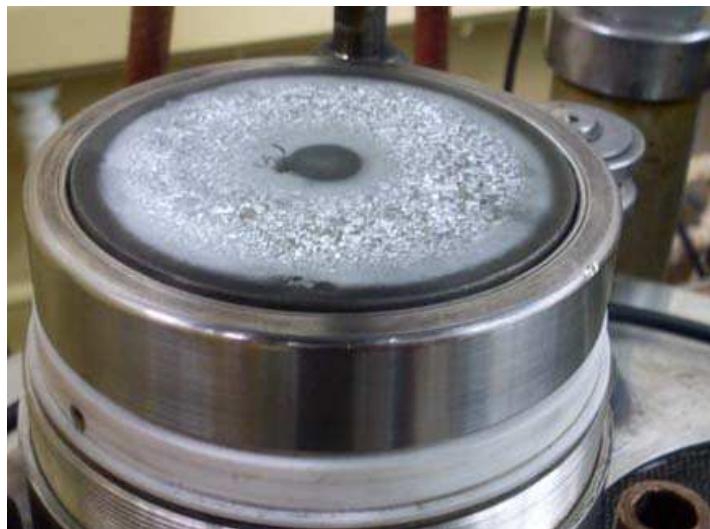
Fig. 2. The zinc target installed on the WMK-100 magnetron
