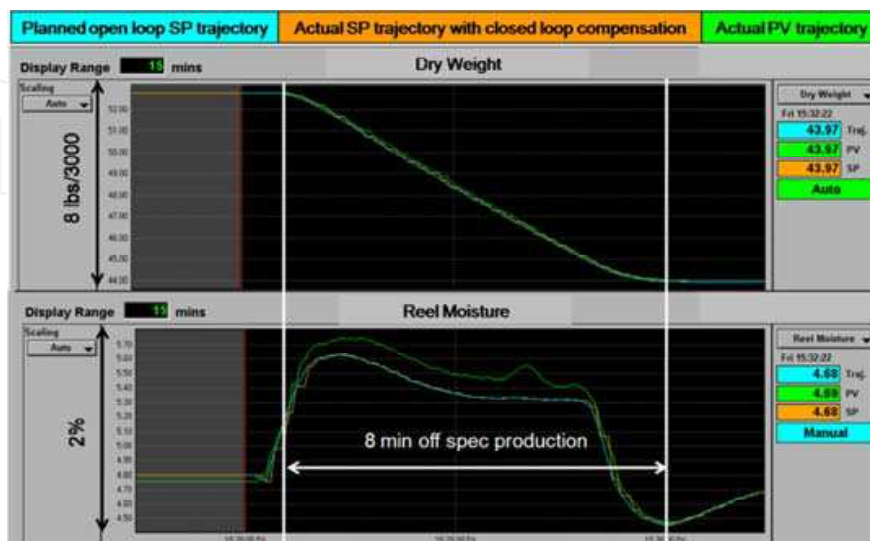
Fig. 15. CV trajectories under closed-loop GC with nonlinear models
