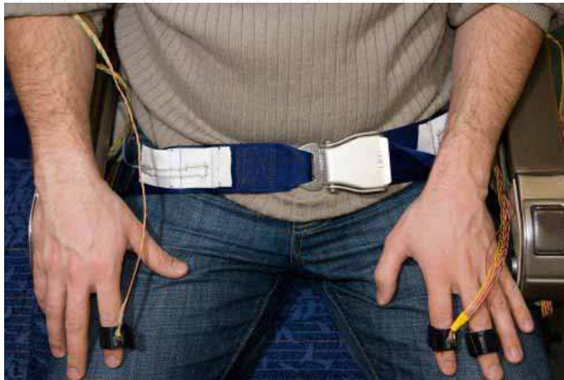
Fig. 7. ECG and EDA measurements at the hand, respiration measurement in the seat belt [Setz et al., 2009]
