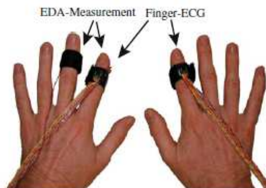
Fig. 2. Combining the measurement of EDA and ECG at the fingers [Schumm et al., 2010]
