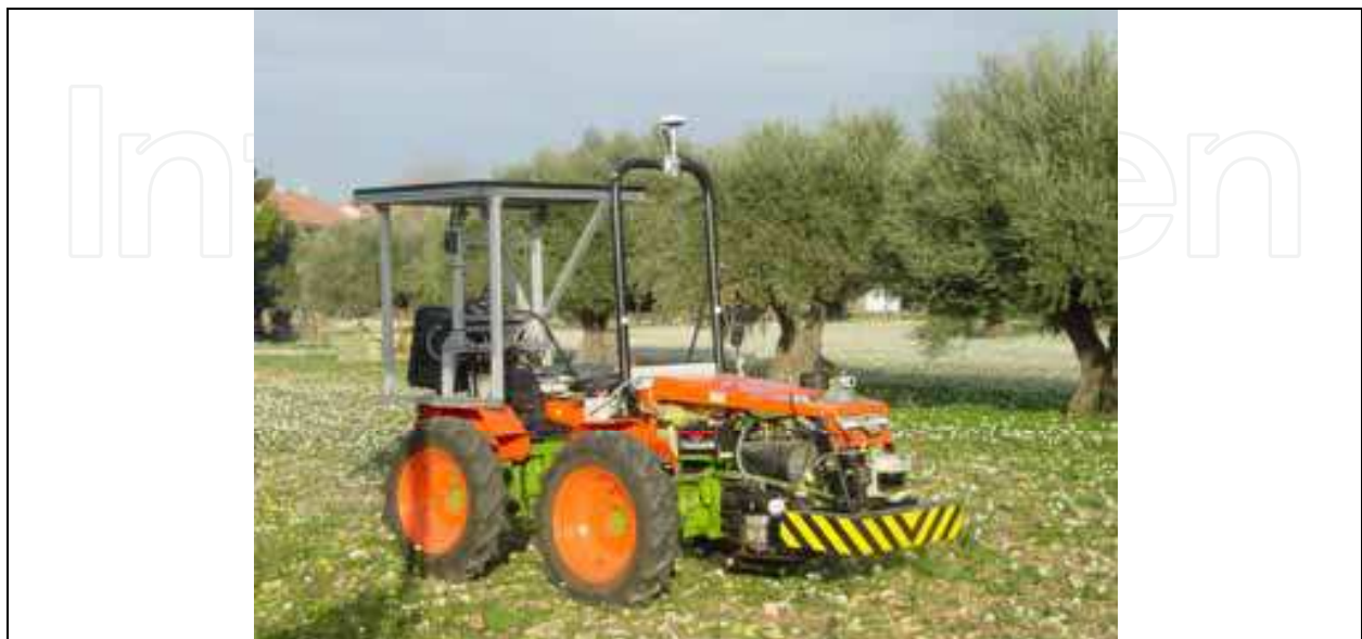
Fig. 1. Experimental vehicle: robot tractor DEDALO
