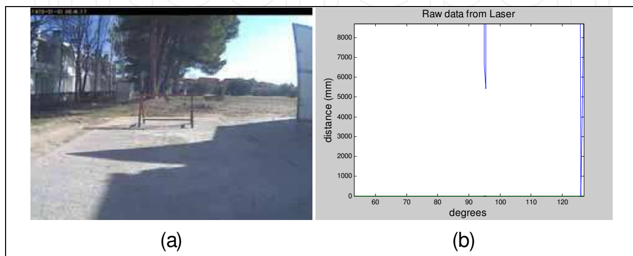
Fig. 8. (a) Visual image displaying the yellow mast on the red sawhorse, (b) Laser image displaying the mast distance.
