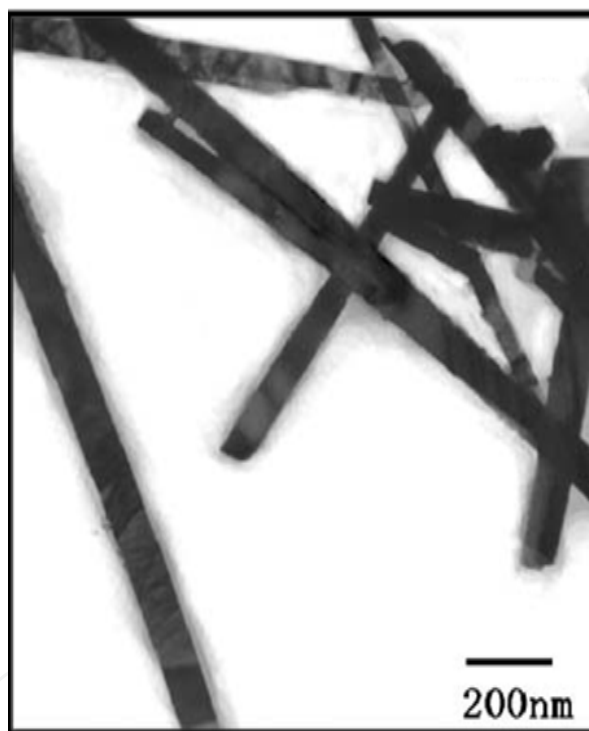
Fig. 2. TEM images of \text{BaCO}_3 obtained by hydrothermal treating for 12 h. [\text{NP}_{10}]=0.127 M and T=140 °C [35]. Reproduced with permission of Elsevier.
