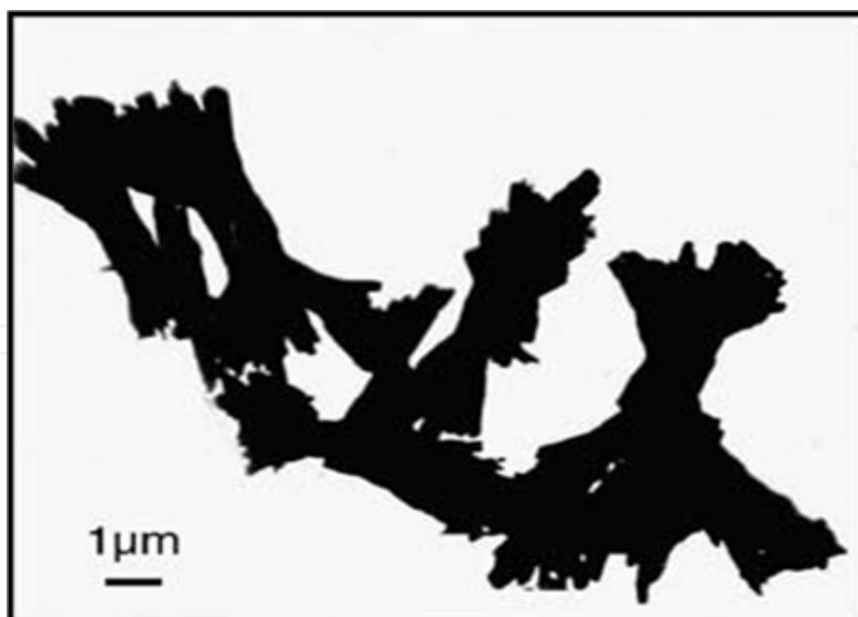
Fig. 4. TEM images of synthesized \text{BaCO}_3 by PVP-assisted method at \text{pH} = 12 [5]. Reproduced with permission of Elsevier.
