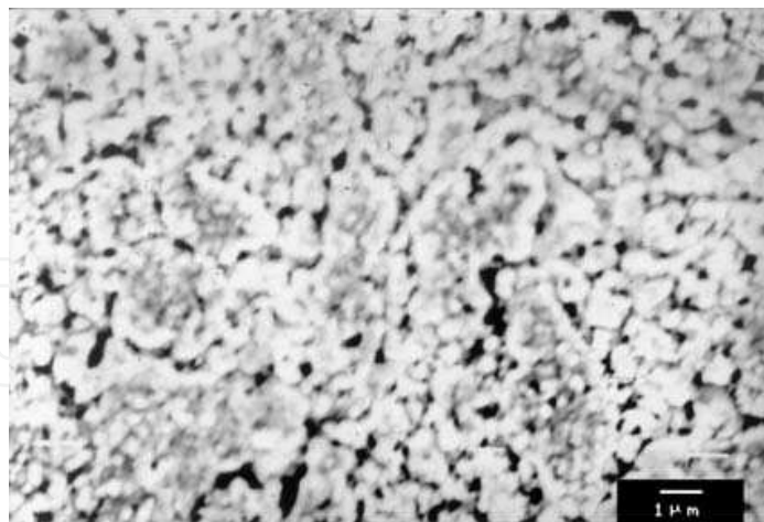
Fig. 10. SEM of the sintered Cu-3wt.%Al 2 O 3 system (900°C, 15 min)
