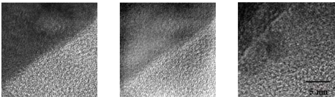
Fig. 16. HRTEM of nanocomposite Cu-5wt.% Al 2 O 3 sintered system
