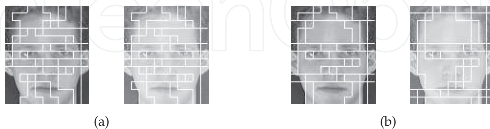
Fig. 35. Viterbi segmentation of face images under different illumination conditions using edge-based feature vectors (a) and DCT-based feature vectors (b); each block corresponds to each state of pseudo-2D HMM.
