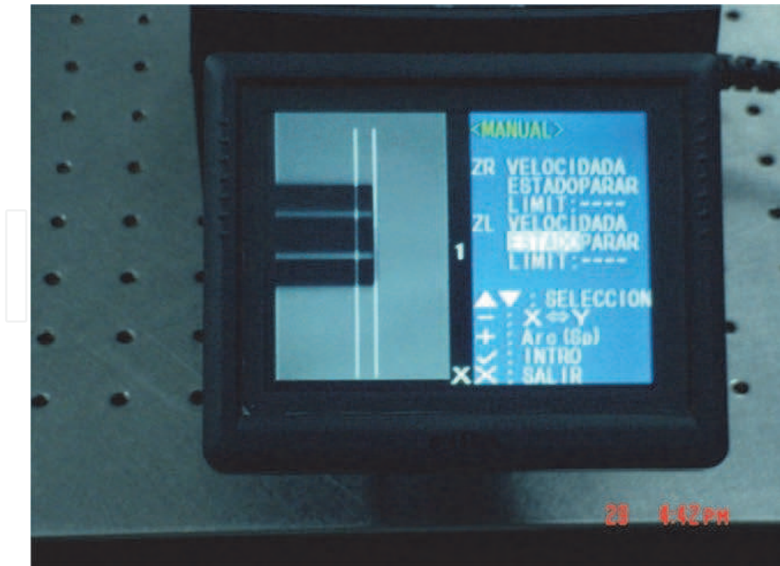
Fig. 2. Application point of the electrical arc (screen on Spanish)
