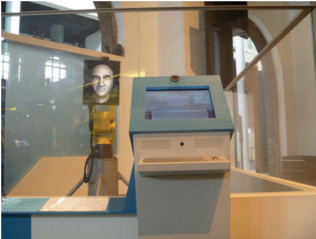
Fig. 7. The information kiosk with the keyboard for language-based interactions with the Articulated Head.
