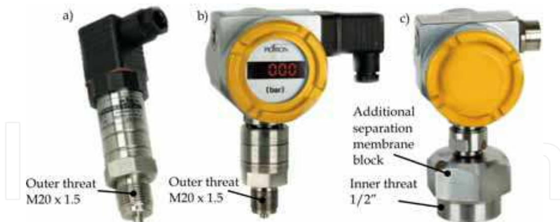
Fig. 3. Examples of commercially available pressure transducers (Peltron, Poland) with stainless steel separation membrane: a) NPX series, b) PXW series with LED display, c) PXC series with additional separation membrane dedicated to harsh environment measurements.
