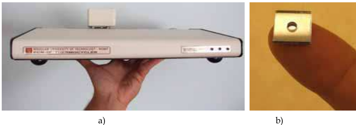
Fig. 37. Desktop real-time PCR device co-working with silicon-glass reusable chips: a) view of the instrument, b) 1 cm x 1 cm chip on author's finger
