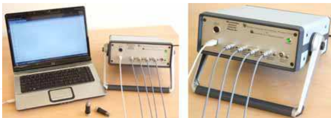
Fig. 16. Commercial-like measurement system driving 5 discrete pressure sensors
