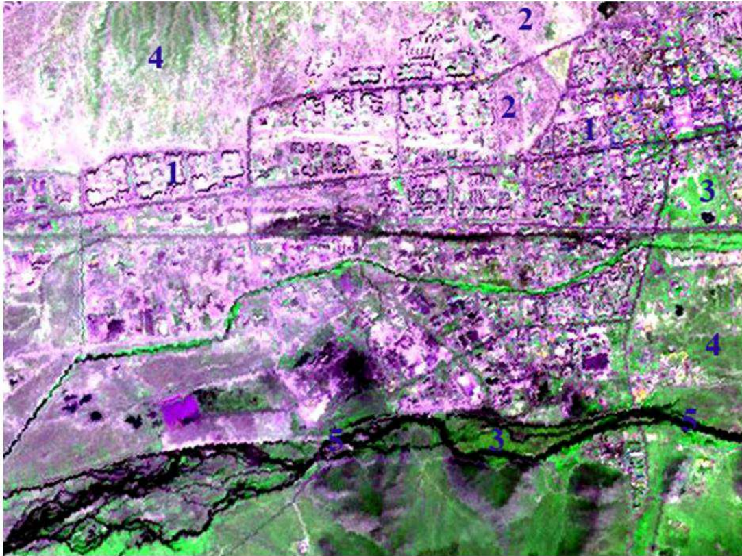
Fig. 1. 2008 ASTER image of the selected part of Ulaanbaatar (B1=B, B3=G, B2=R). 1-built-up area; 2-ger area; 3-green area; 4-soil; 5-water. The size of the displayed area is about 8.01kmx6.08km.
