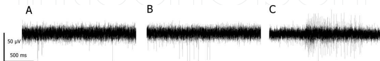
Fig. 2. Development of signalling in MEA. (A) First, after the neuronal cells have grown few days on MEA, first signals are detected. They are individual single spikes. (B) Then, about after 1-2 weeks of culturing spiking activity matures into training phase. There are several spikes organised together. (C) Finally, bursting activity occurs. Burst is a complex signal package that happens in several channels at the same time.
