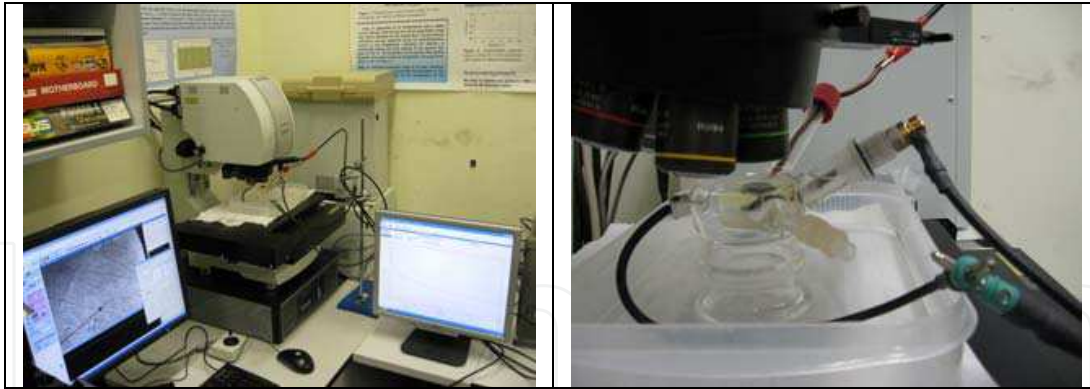
Fig. 9. Photographs of the minicell placed in the CLSM.
