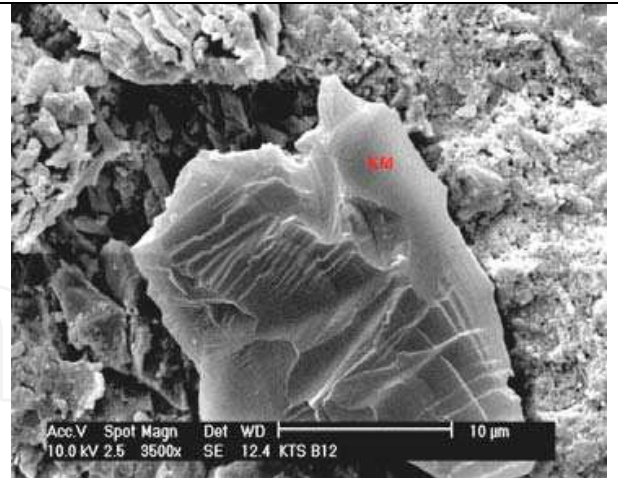
Fig. 16. Alkalifeldspar with typical twinning structure with calc as well as salt recrystallization.
