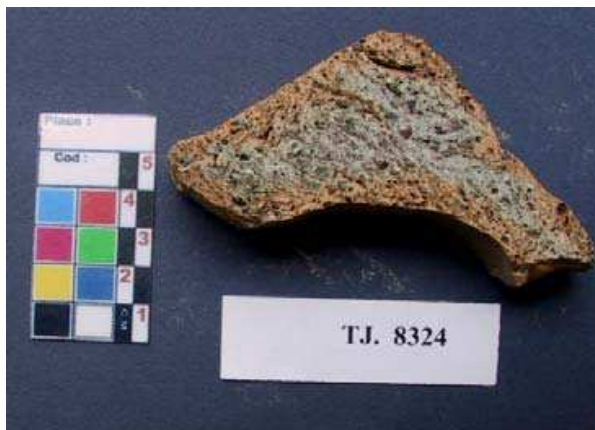
Fig. 1. Ceramic with different colors in the matrix as a function of uncontrolling firing.
