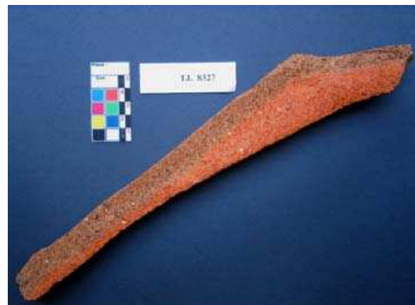
Fig. 2. A part of a Vase structure varies from the surface to the core and also different admixtures
