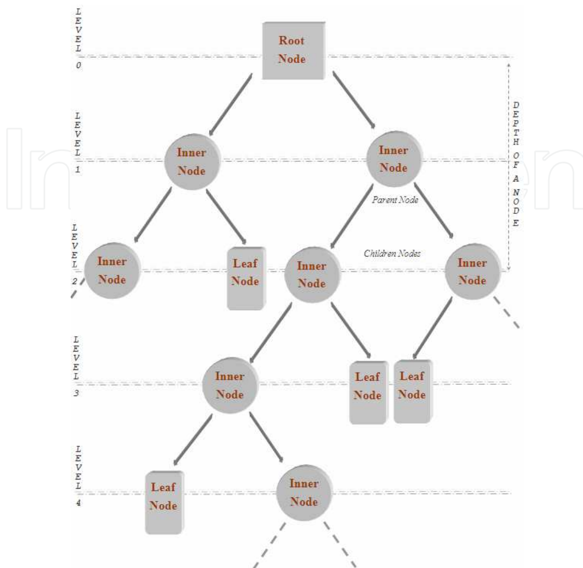
Fig. 13. In computers, knowledge can be represented as binary trees, consisting of a root node, inner nodes and leaves
