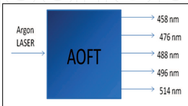
Fig. The AOTF enables you to select the wavelengths (laser lines on/off)
