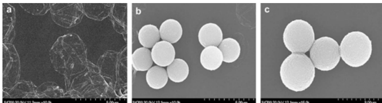
Fig. 10. SEM images of the (ALG/CHI) 5 hollow shells (a) and shells upon incubating the preformed shells in various organic solutions in pure water medium: (b) DCP; (c) SA. Scale bars are 5 mm for a, 5 mm for b and 3 mm for c. (Ding et al., 2009)
