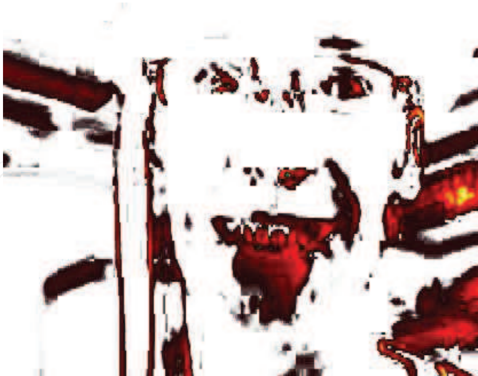
Fig. 3. Variance for the individual pixels in a video sequence. White = low variance Yellow = high variance
