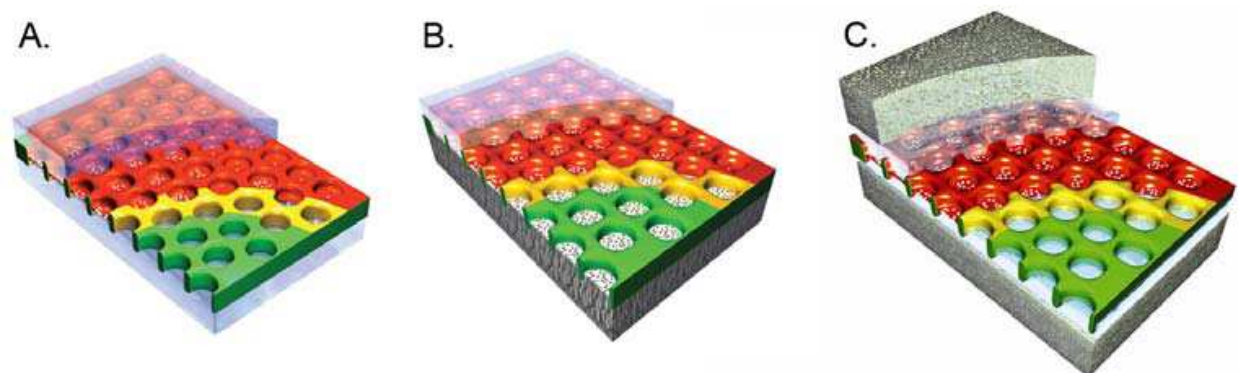
Fig. 1. Biomimetic membrane array designs using micro-structured ethylene tetrafluoroethylene (ETFE) as scaffold. A) ETFE membrane scaffold for freely suspended planar membrane arrays. B) Composite half-sandwich membrane scaffold consisting of an ETFE partition partly embedded in a porous support structure to create individually well-defined wells (grey). C) Complete composite scaffold sandwich structure. Shown in the illustrations are the ETFE membrane scaffold (green), surface modifications of the ETFE scaffold (yellow), biomimetic membranes (red), proteins (white), aqueous layers or hydrogel polymers (transparent) and porous supportive structures (grey).
