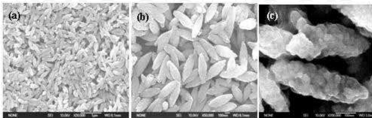
Fig. 10. SEM micrographs of \text{SrCO}_3 prepared using (\text{NH}_4)_2\text{CO}_3 and \text{Sr}(\text{NO}_3)_2 by microwave heating at 90 °C for 5 min in ethylene glycol. Reproduced with permission from J. Nanosci. Nanotechnol. 2007, 7, 4552. Copyright 2007 ASP.
