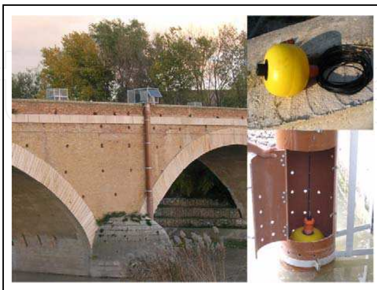
Fig. 2. The suspended sediment measuring station and the optical device (instrument).
