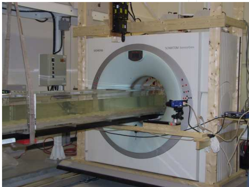
Fig. 1. CT-scanner gantry moving along the flume on four parallel rails and open-channel flume fixed on the examination table.
