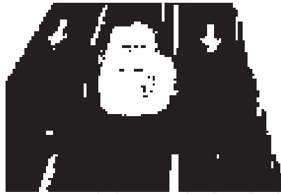
Fig. 4. Binary image obtained by a 2-cluster segmentation. The white blob is the vehicle in motion and the white vertical stripes are divisions of the lanes.
