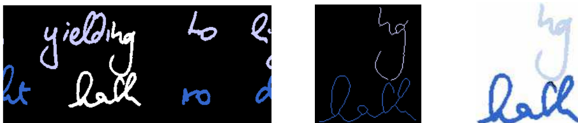
Fig. 6. Segmentation of a CC running along two text lines (reprinted from Papavassiliou et al., 2010).
