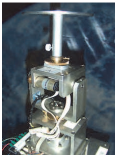
Fig. 2. Rotational motion simulator using z-y-z Euler angles.
