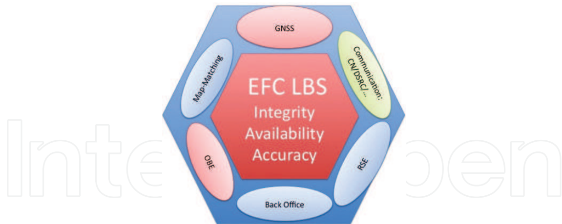
Fig. 1. Several elements comprise a GNSS-based electronic fee collection system.
