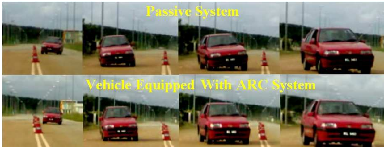
Fig. 34. Visual comparison of experimental results between passive system and vehicle equipped with ARC system during double lane change test
