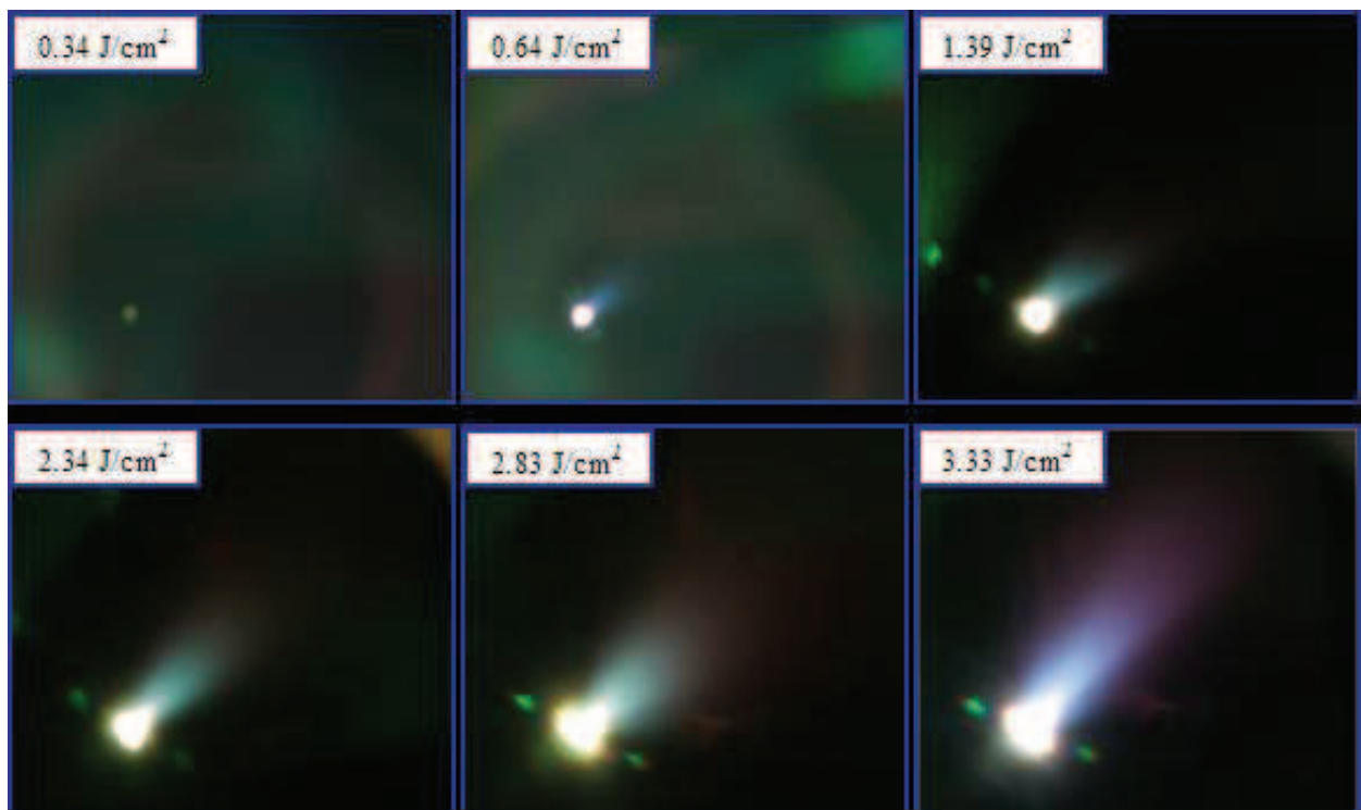
Fig. 3. CdS plume pictures at different laser fluences. Plasma is seen around 0.64 \text{ J/cm}^2 indicating the threshold of the ablation fluence
