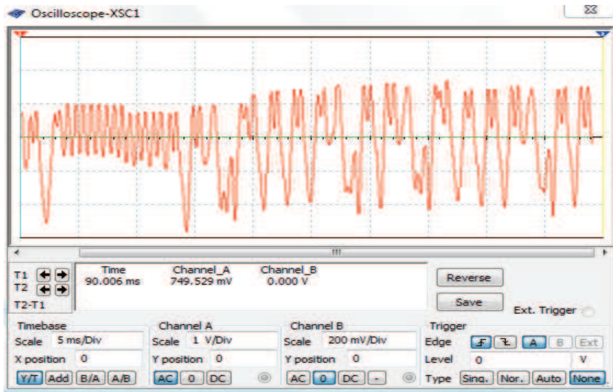
Fig. 17. For R_1=6\text{K}\Omega , the voltage signal and LED response are chaotic
