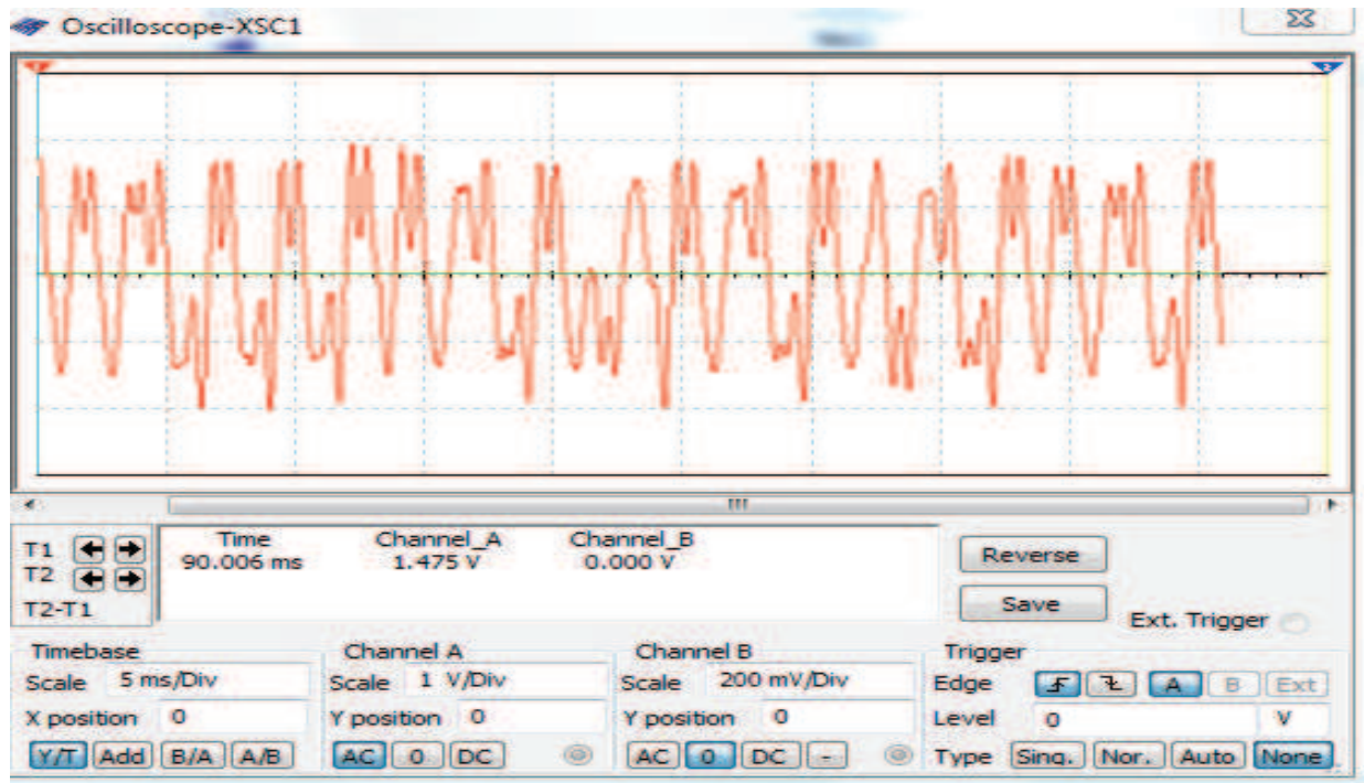
Fig. 18. For R_1=6.81K\Omega the voltage signal and LED response are chaotic
