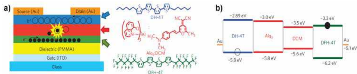
Fig. 10. Tri-layer device structure along with chemical structures of the organic materials used for the device fabrication (a), HOMO and LUMO energetic levels of the materials (b)
