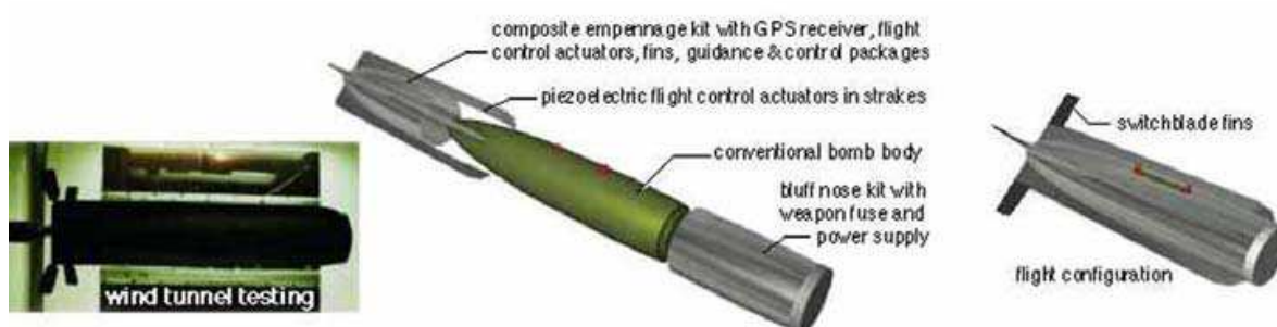
Fig. 8. Smart Compressed Reversed Adaptive Munition (SCRAM) 19,20
