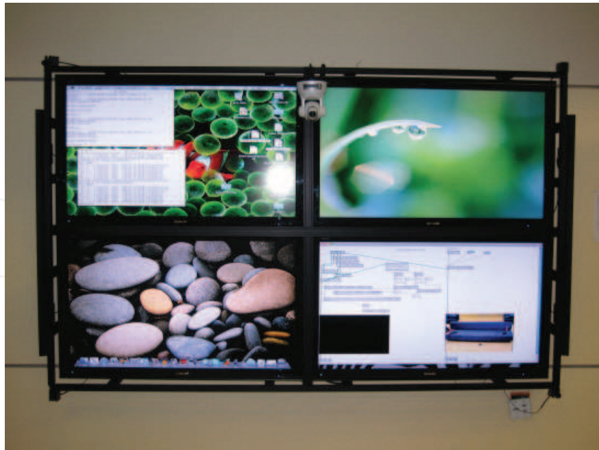
Fig. 1. Frontal view of TAC display unit. PTZ camera and four of the seven total microphone are visible.
