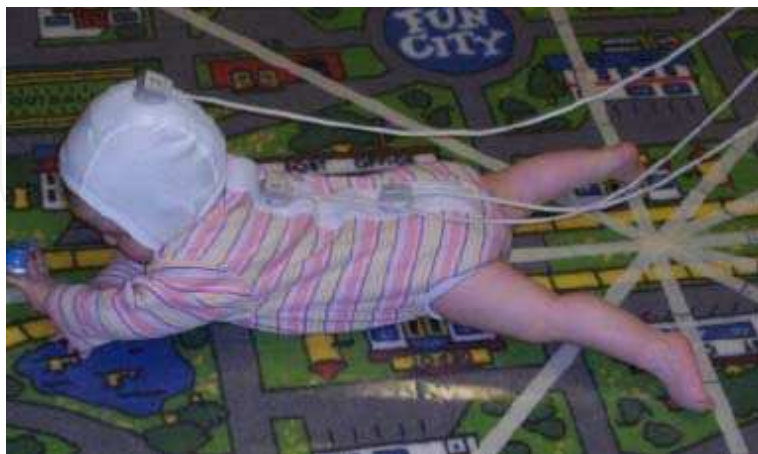
Fig. 9. A 7-month-old infant wearing a special body and hat placed prone in the rotation circle and participating in the experiment. The magnetic trackers to measure the infant's rotation movements were placed on the head, between the shoulder blades, and on the lower back.
