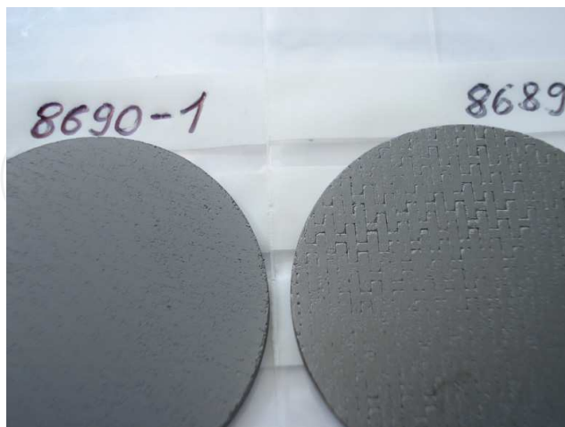
Fig. 9. Pictures of two CVDed SiC coated C/SiC specimens obtained by physical vapour infiltration.
